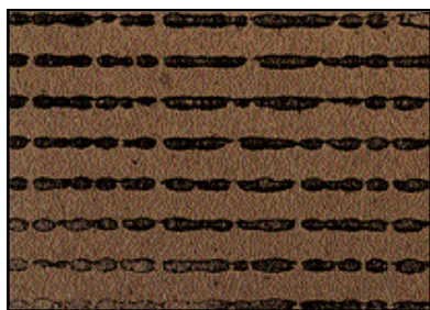
GLUE APPLICATION FROM A CONVENTIONAL GLUE MACHINE*
