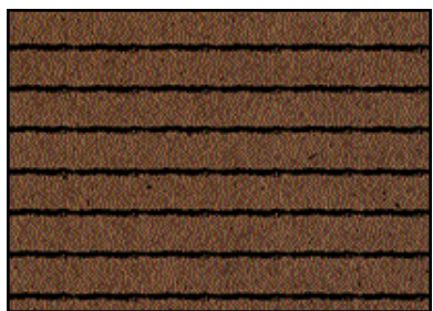
GLUE APPLICATION FROM AN ISO-BAR GLUE MACHINE
